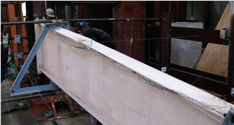
Test of rafter showing the formation of lateral torsional buckle.
