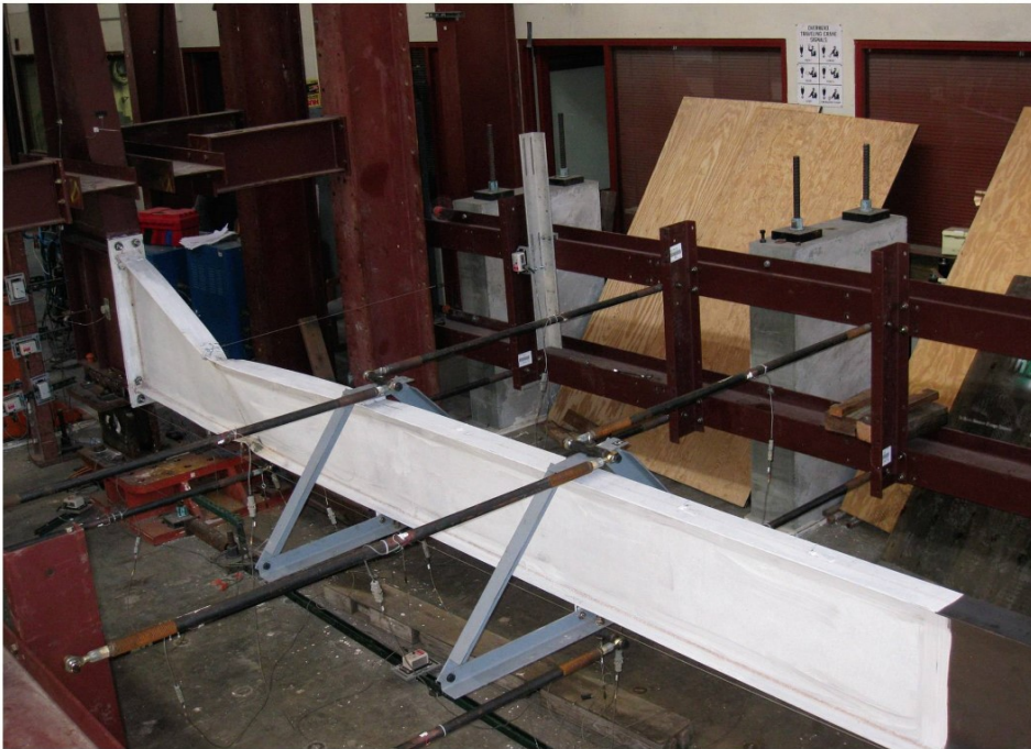
Photo 4: One of the series of tests performed at UCSD, subjecting a partial frame of tapered members to a cyclic load, to observe the buckling behavior.
