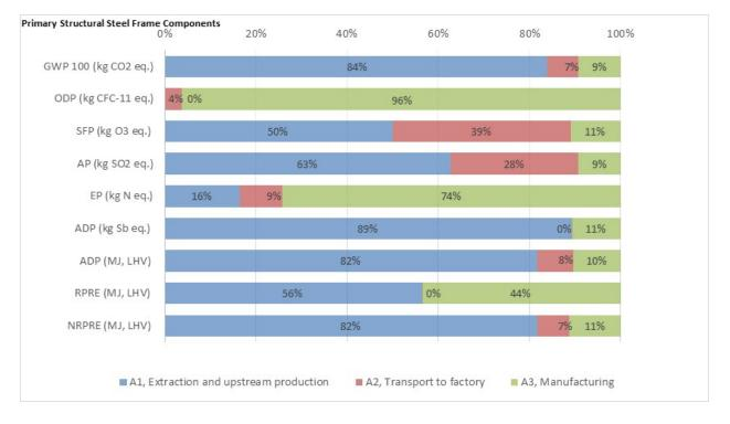
Figure 7 Impact assessment and energy indicator results by stage – 1 metric ton of primary frame – % Basis
