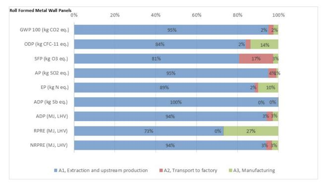
Figure 9 Impact assessment and energy indicator results by stage – 100  $m^2$  of wall panels – % Basis
