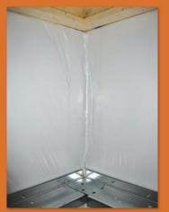
This corner detail, as built in the laboratory, is ready for air leakage evaluation. Careful detailing of the corner joint yields valuable information about improving the detail design.
