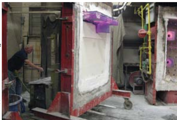
The wall and HOW assembly successfully passed the fire test. Photo courtesy of MBMA.
