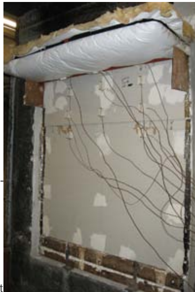
The fire resistant wall and Head-of-Joint assembly being tested at Underwriters Laboratories. Photo courtesy of MBMA.
