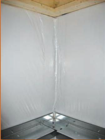
This corner detail, as built in the laboratory, is ready for air leakage evaluation. Careful detailing of the corner joint yields valuable information about improving the detail design.
