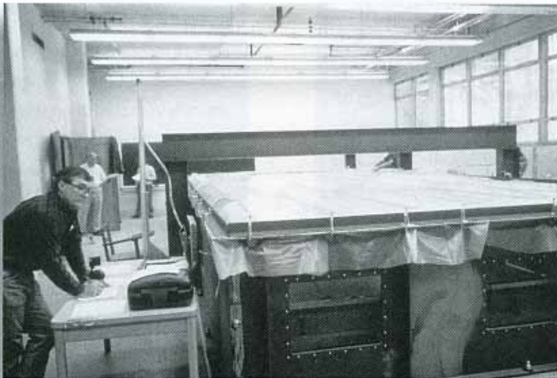
Photo 5: ASTM E1592 test of a standing seam roof to determine uplift capacity.
