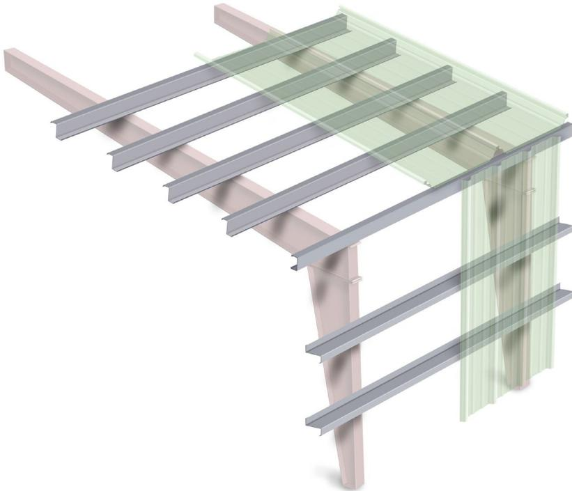
Illustration of secondary structural steel framing (girts/purlins) supporting the metal roof panel (standing seam or through fastened) and metal wall panel (through fastened) cladding. The girts and purlins are attached to the primary structural steel framing.
